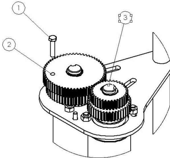
If the bolt (1) is fitted in position 2, the top set of gears provide the stretch (70%).
