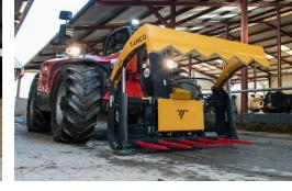
[01] The i74 Meal Bucket is locked to the BaleShear with a pin connected to the gripping mechanism, making collection and drop-off of the bucket simple and without the need to exit the cab, saving time.
