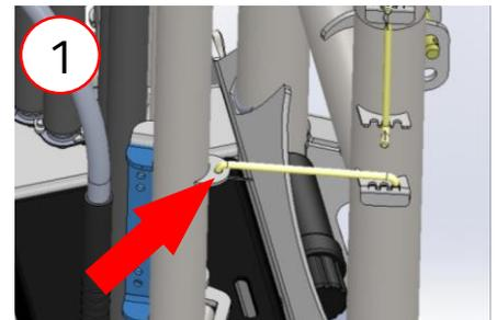
2. Position the safety arms into the working position by removing the retaining pin.
