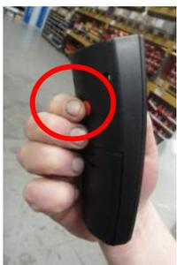
The red button on the rear of the remote must be pressed while pressing any other button (except "STOP").
