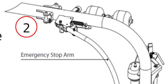
3. Adjust the load arm stop pin to allow clearance between the top of the bale at the rotating arm.
