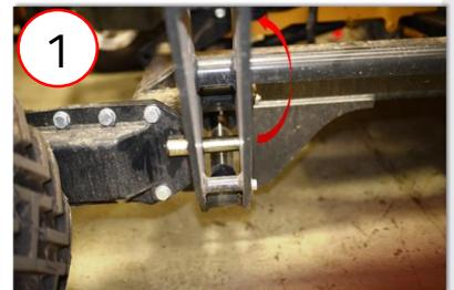
2. Adjust the load arm width to suit the correct bale size.
