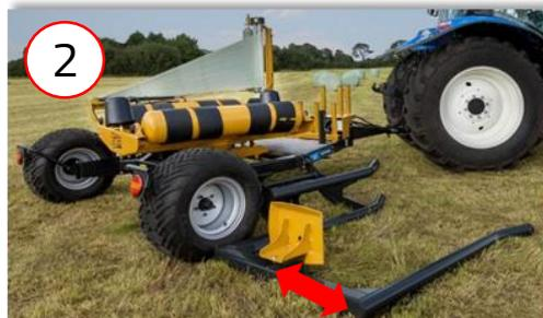
3. Adjust the position of the dispenser to ensure that the film will be applied to the centre of the bale.
