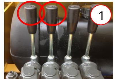
2. Remove the transport bracket and lower the unloading conveyor to the ground.
